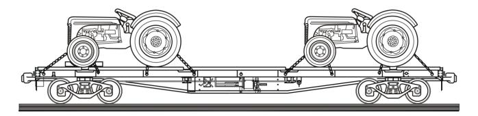
12. You will note that they have been positioned so that the front wheels of one tractor and the rear wheels of the other tractor have been positioned over the center of the bogie bolsters.
